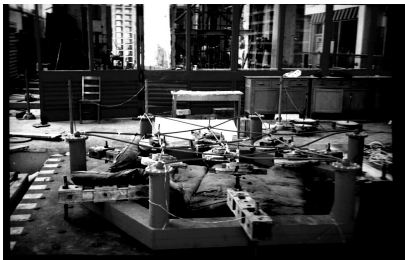
Fig. 8. Photo of global dynamic instability of Model 2.
